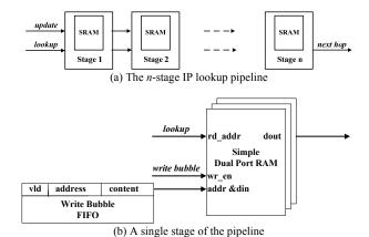
Figure 3. The SRAM-based IP lookup pipeline
