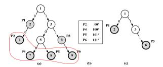
Figure 1. (a) A sample trie, (b) the corresponding disjoint prefix set, and (c) the corresponding overlapping prefix set (a small trie).
