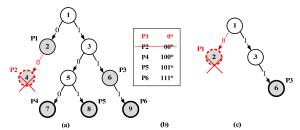
Figure 5. (a) Deletion of an existing prefix, (b) its corresponding disjoint prefix set, and (c) its corresponding overlapping trie
