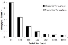
Figure 10. The throughput of the hybrid architecture
